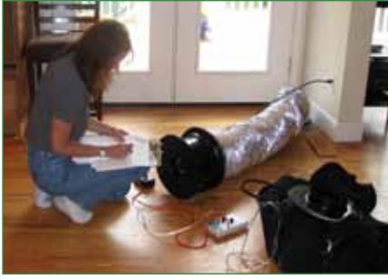
Energy Expert Cathy Cartmill tests a home's duct system. Leaky ductwork can increase heating & cooling costs and cause indoor air quality problems.
